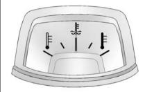
This gauge shows the engine coolant temperature.
