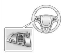
n: Press to turn the system on and off. A white indicator appears in the instrument cluster when cruise is turned on.
