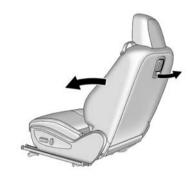
To access the rear seats, pull up on the latch on the rear of the driver or front passenger seatback. Fold the backrest forward.
