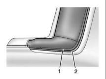
Push the outside rim (1) of the tonneau cover under the vehicle trim (2) on both sides.
