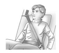
Buckle, position, and release the safety belt as described previously in this section. Make sure the shoulder portion of the belt is on the shoulder and not falling off of it. The belt should be close to, but not contacting, the neck. To remove and store the comfort guide, squeeze the belt edges together so that the safety belt can be removed from the guide. Slide the guide onto the clip, leaving only the loop of the elastic cord exposed.
