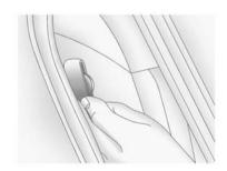
Pull the elastic cord out from between the edge of the backrest and the interior body to remove the guide from its storage clip.
