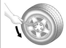
Use the fully extended wheel wrench to loosen all the wheel nuts one-half turn counterclockwise. Do not remove them yet.
