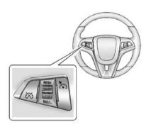
ৈ (On/Off): Press to turn the system on and off. A white indicator appears in the instrument cluster when cruise is turned on.
