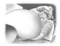
The front outboard passenger frontal airbag is in the instrument panel on the passenger side.
